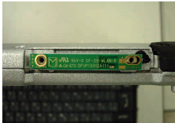
Send & Receive Antenna View
