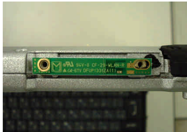
Send & Receive Antenna View
