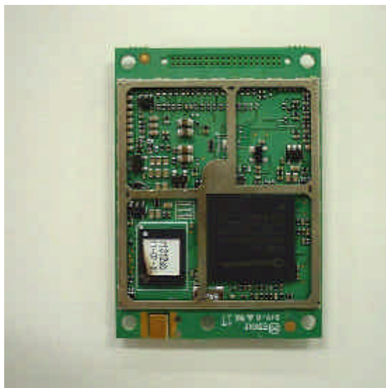
SB555 Module Interior Top View
