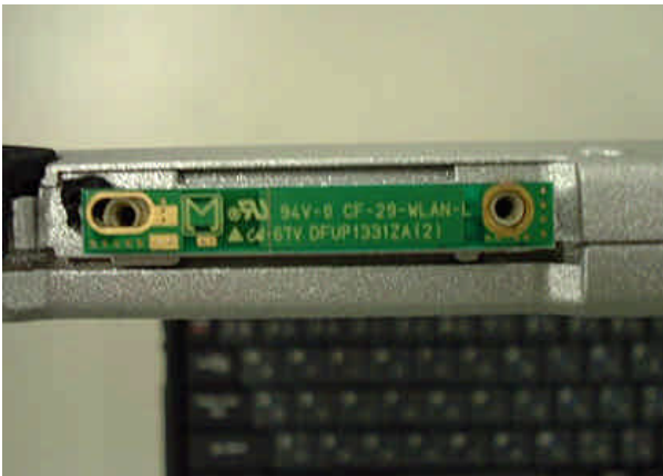
Receive only Antenna View
