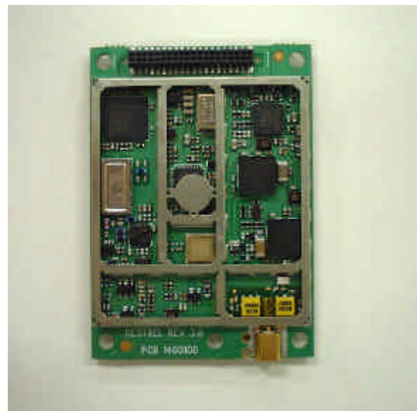
SB555 Module Interior Bottom View
