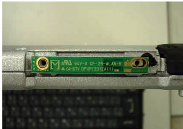
Send & Receive Antenna View
