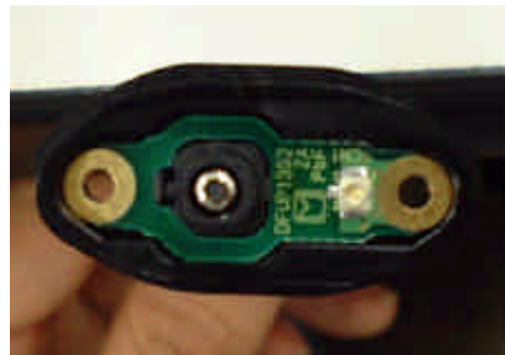
Whip Antenna I/F PWB
