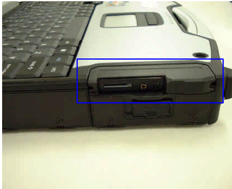
SB555 Module Adapter Position
