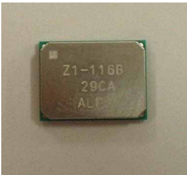
Top View of Bluetooth Module
