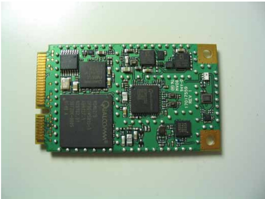
HSDPA Module Interior Bottom View
