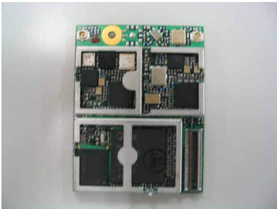
EM5625D Module Interior Bottom View
