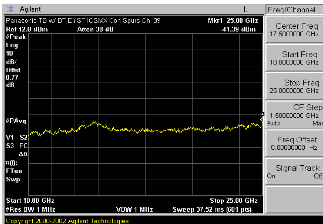
Plot 6-13. Conducted Spurious Plot (Bluetooth – Ch. 39)
