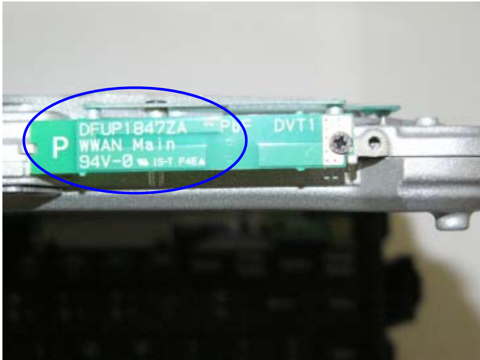
WWAN Main TX/RX Antenna
