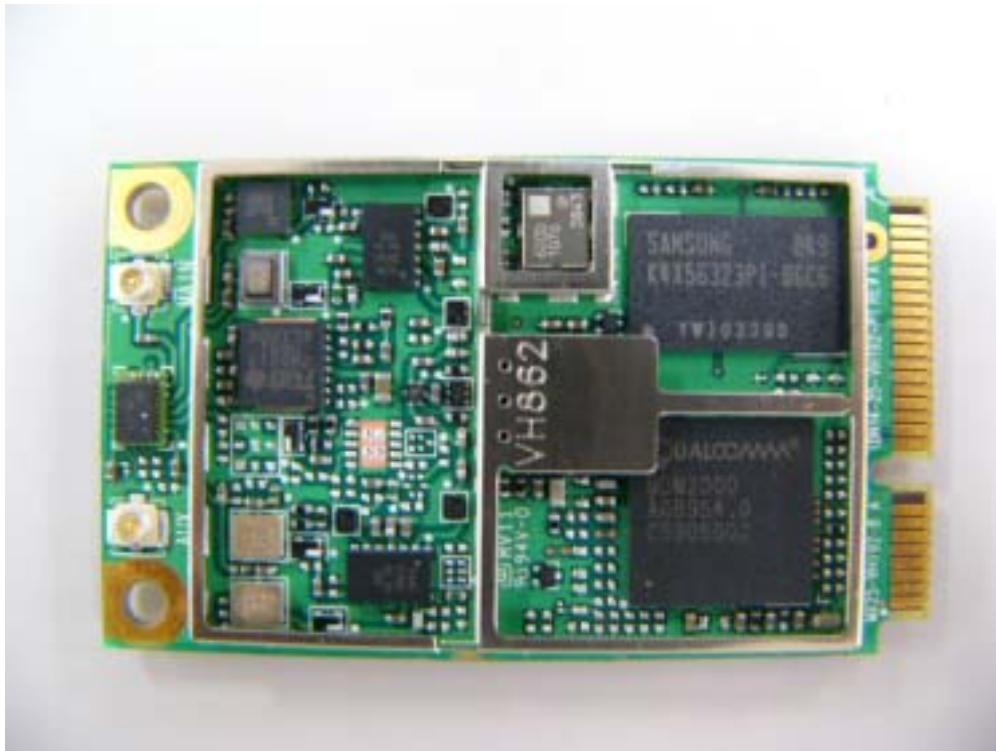
WWAN Module Interior Top View
