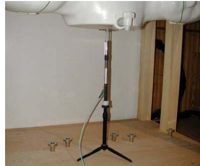
Figure 12-2 System Verification Setup Photo
