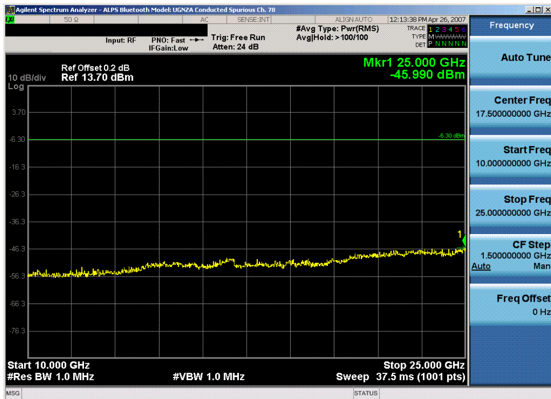
Plot 6-17. Conducted Spurious Plot (Bluetooth – Ch. 78)
