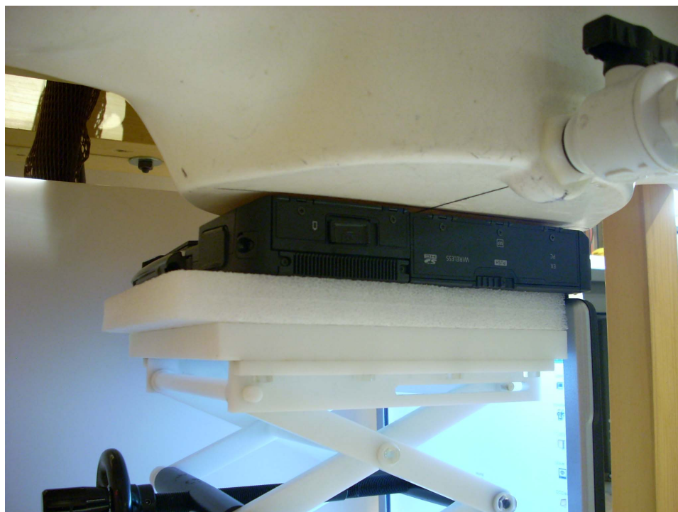
Figure 19-2 SAR Test Setup Photo 2 (Lap Position)
