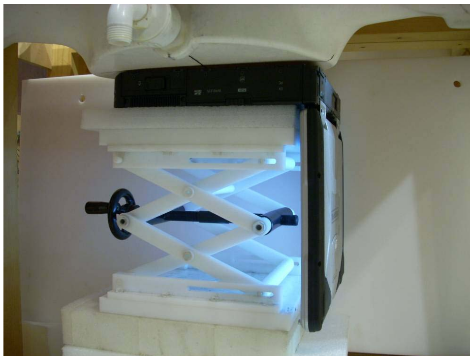
Figure 19-1 SAR Test Setup Photo 1 (Lap Position )
