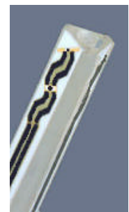
Figure 3.2 Probe Thick-Film Technique
