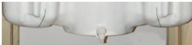
Figure 7.2 SAM Twin Phantom shell
