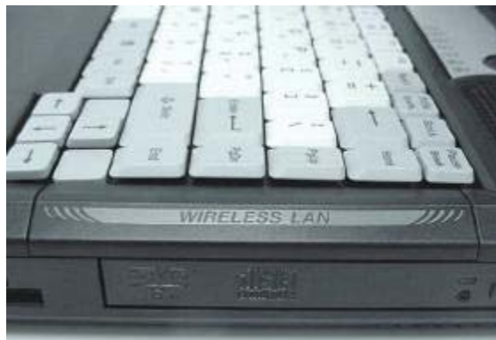
Location of Internal Antenna 1 (A0)
