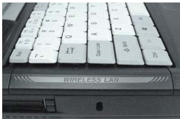
Location of Internal Antenna 2 (A1)
