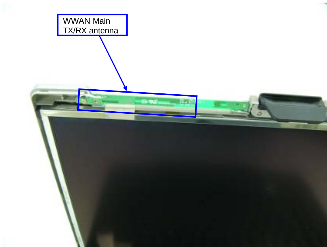
WWAN Main TX/RX Antenna
