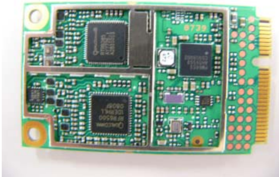
WWAN Module Interior Bottom View
