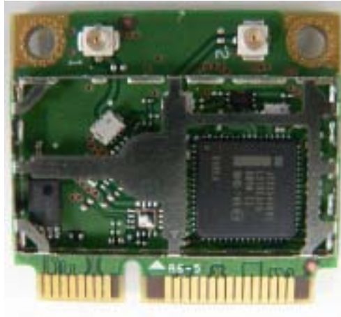
WLAN inside Top View
