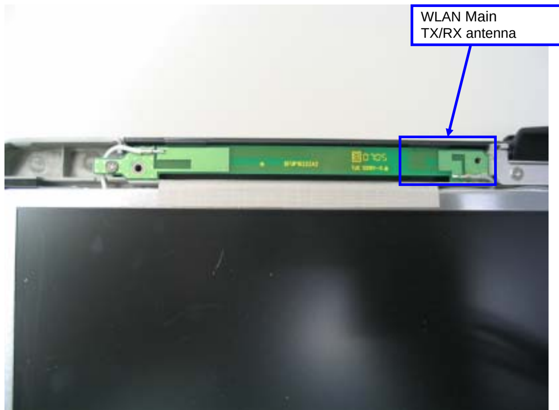
WLAN Main antenna magnified view
