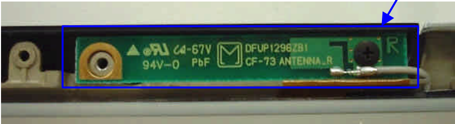
Send & Receive Antenna View
