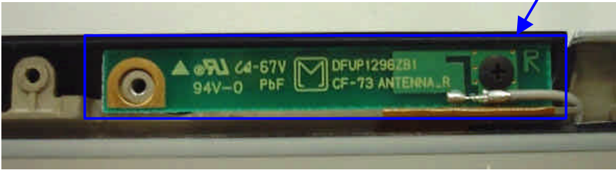
Send & Receive Antenna View
