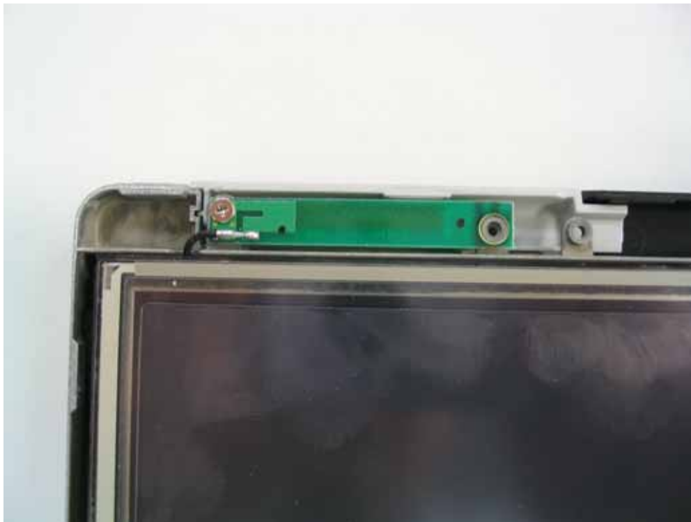
WLAN Main antenna magnified view
