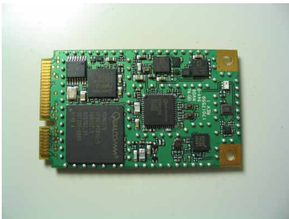
HSDPA Module Interior Bottom View
