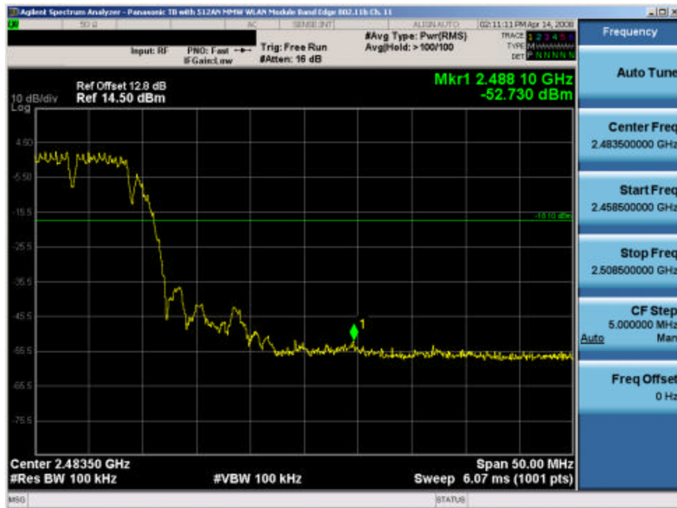
Plot 6-30. Band Edge Plot (802.11b – Ch. 11)
