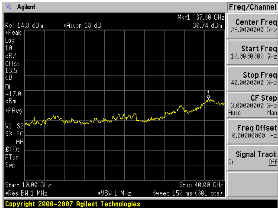
Plot 6-46. Conducted Spurious Plot (802.11a – Ch. 149)
