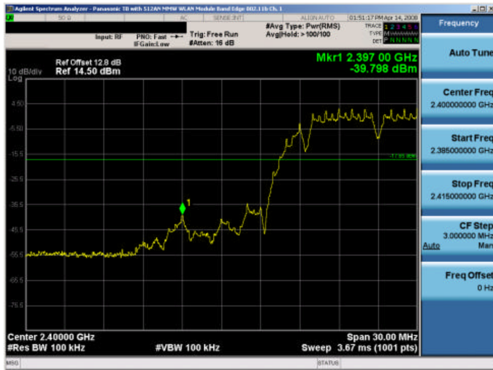
Plot 6-29. Band Edge Plot (802.11b – Ch. 1)
