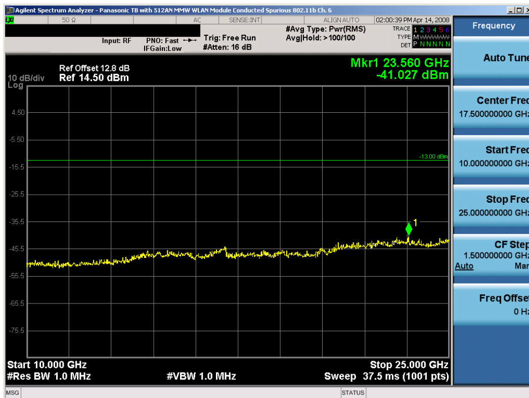
Plot 6-42. Conducted Spurious Plot (802.11b – Ch. 6)
