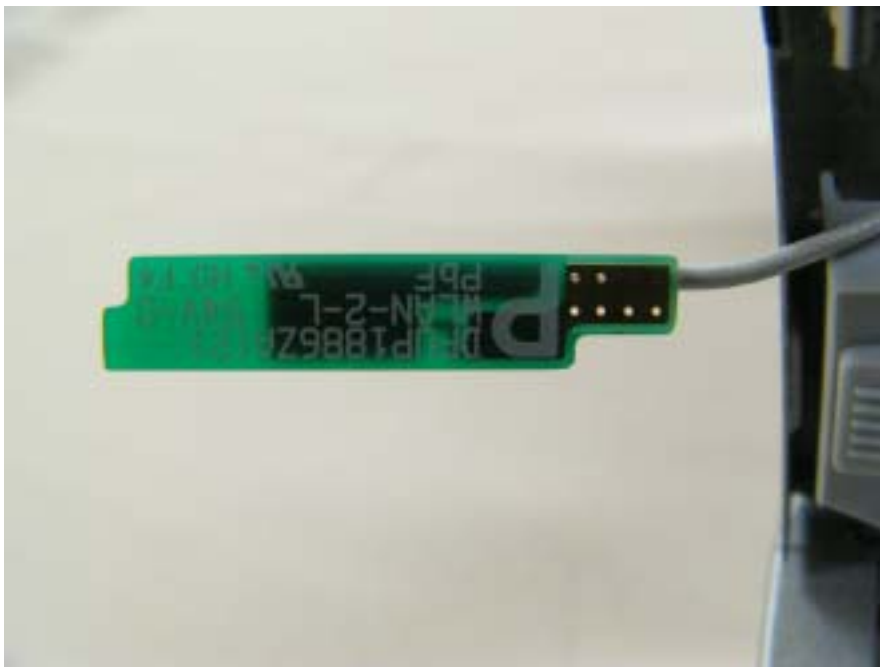
WLAN Aux TX/RX antenna magnified view (Top)
