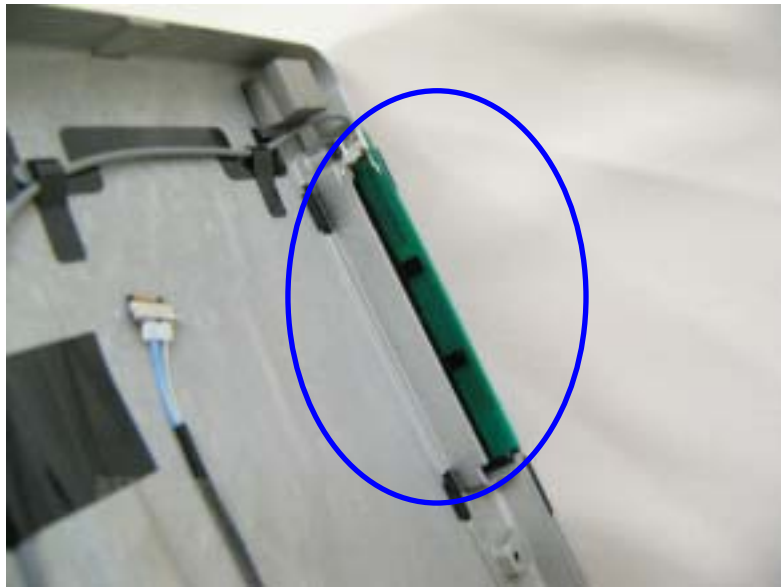
WWAN Main TX/RX Antenna
