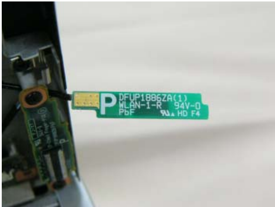
WLAN Main TX/RX antenna magnified view (Top)
