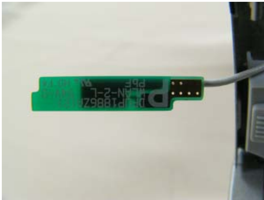
WLAN Aux TX/RX antenna magnified view (Top)
