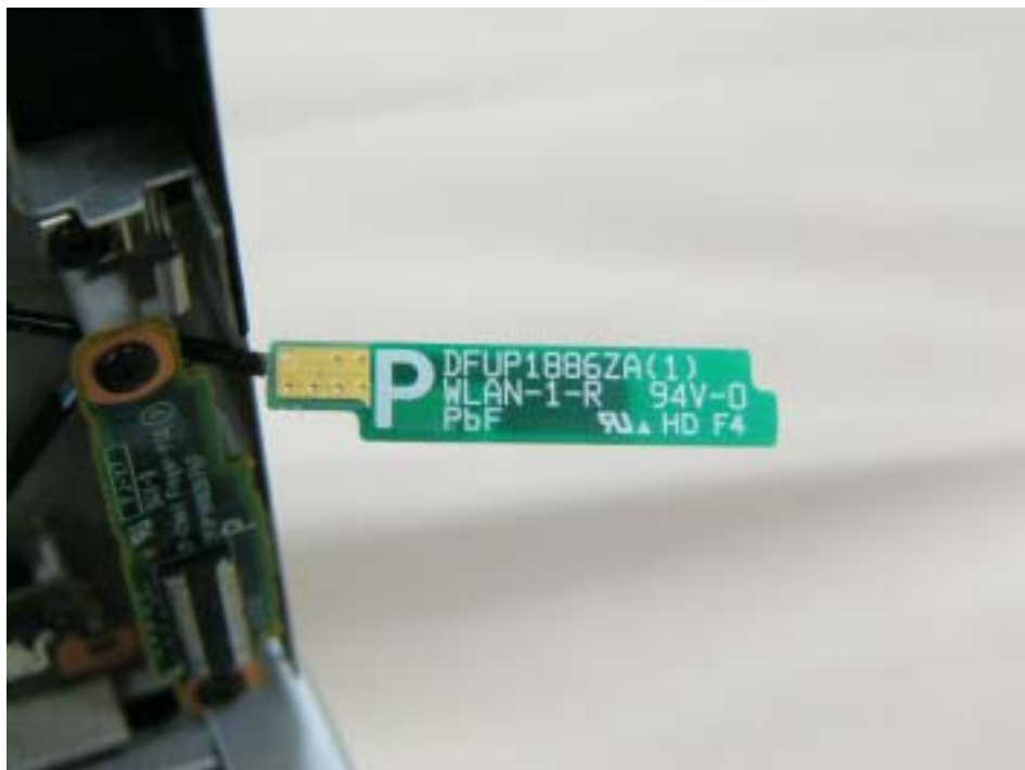
WLAN Main TX/RX antenna magnified view (Top)
