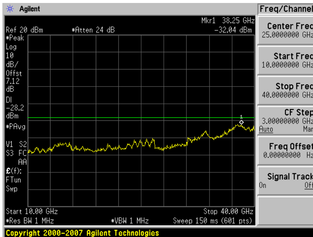
Plot 6-73. Conducted Spurious Plot (802.11a – Ch. 157) – Chain B
