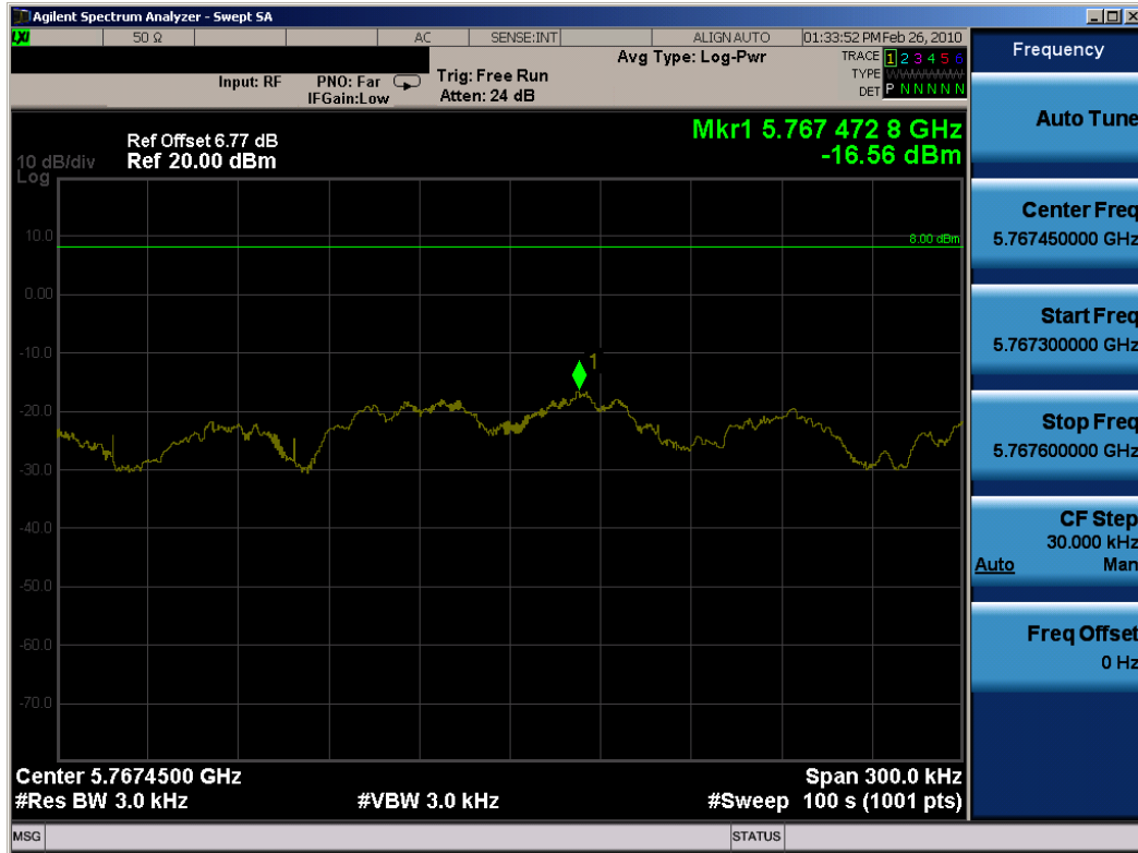
Plot 6-27. Power Spectral Density (802.11n (5.8GHz) Dual Transmit Mode – Ch. 151) – Chain A
