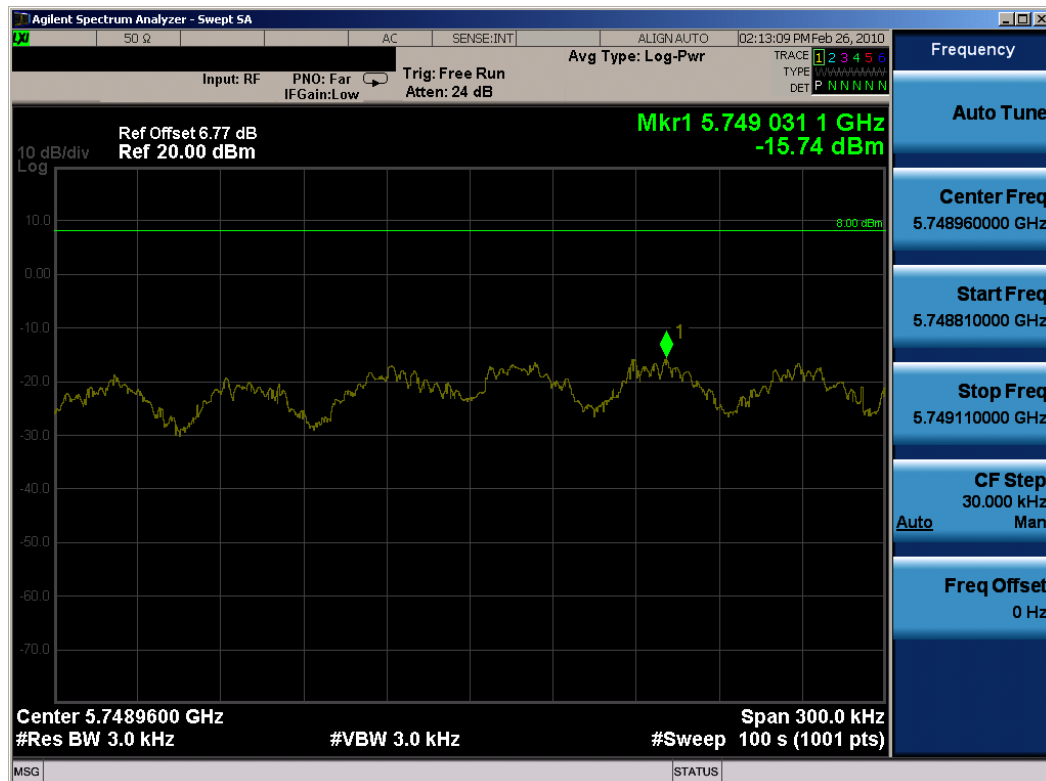
Plot 6-24. Power Spectral Density (802.11a Dual Transmit Mode – Ch. 149) – Chain B
