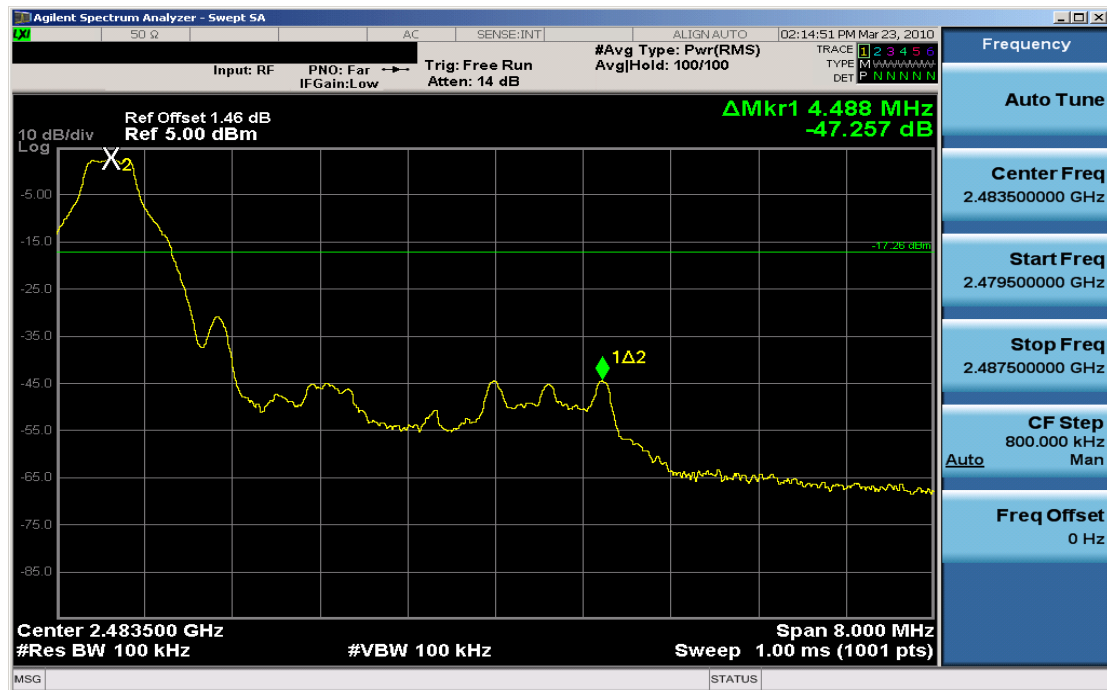
Plot 6-5. Band Edge Plot (Bluetooth – Ch. 78)
