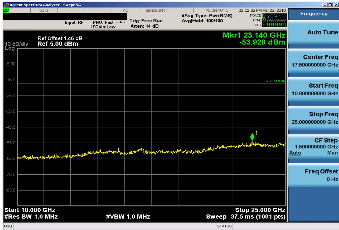
Plot 6-13. Conducted Spurious Plot (Bluetooth – Ch. 0)
