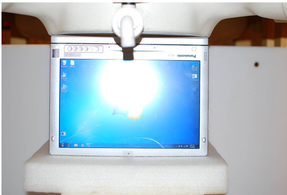
Figure 19-4 SAR Test Setup Photo 4: Edge Bottom
