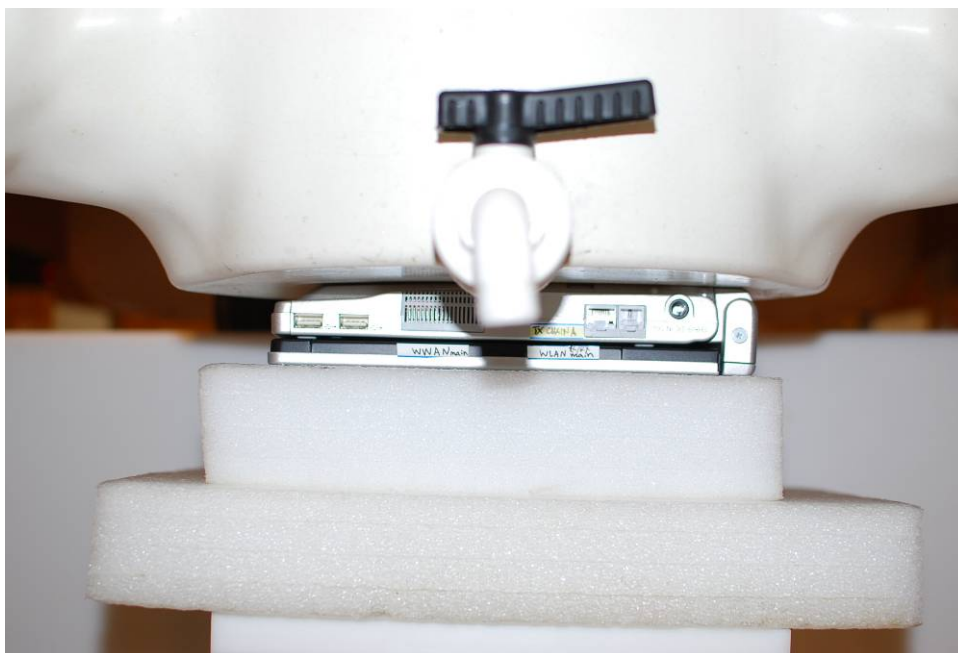
Figure 19-2 SAR Test Setup Photo 2: Laptop WLAN Antenna A, WWAN Antenna (Right)
