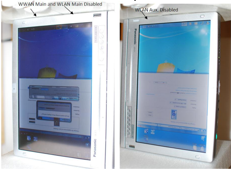
Figure 19-5 Antenna Function and Screen Rotation
