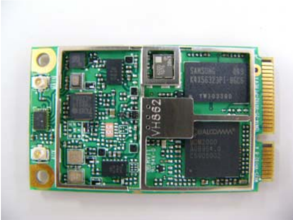
WWAN Module Interior Top View
