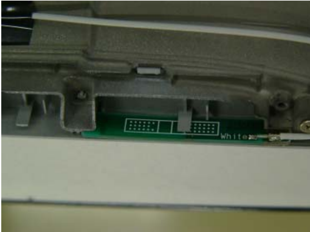
WWAN MAIN TX/RX Antenna
