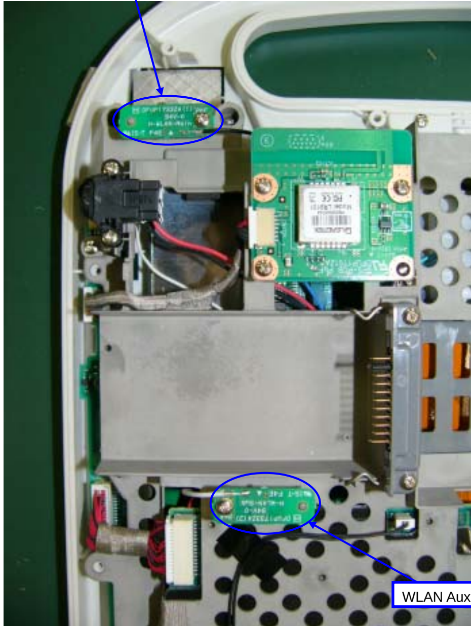
WLAN Main TX/RX Antenna & WLAN Aux RX Antenna
