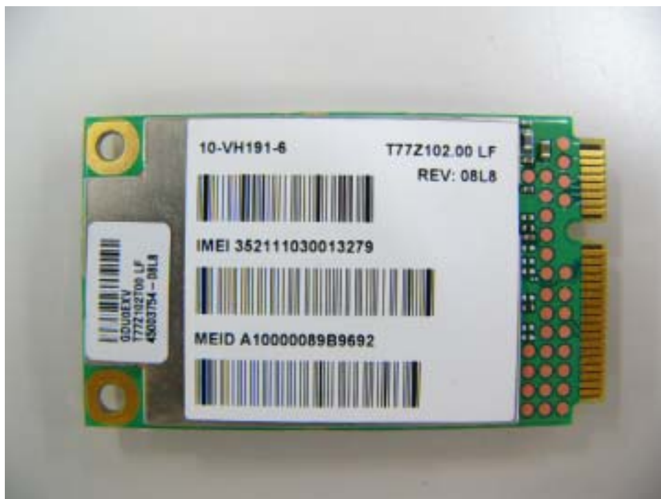
WWAN Module Bottom View
