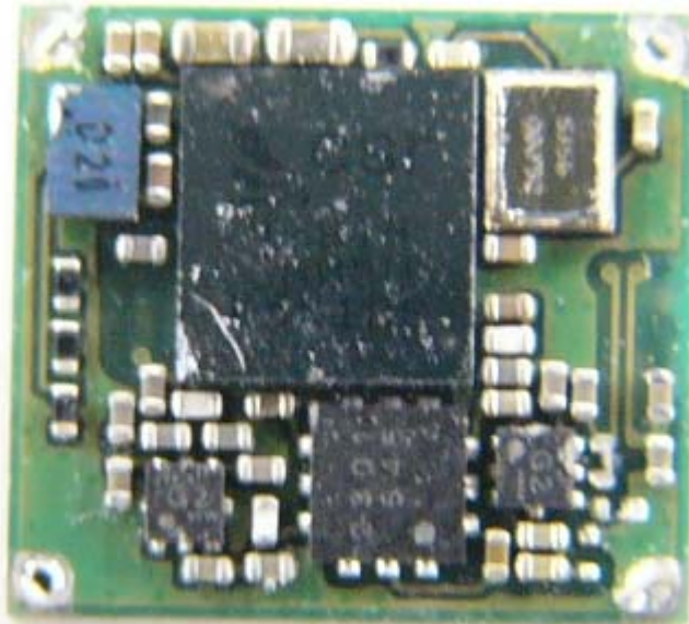
Bluetooth Module inside Top View
