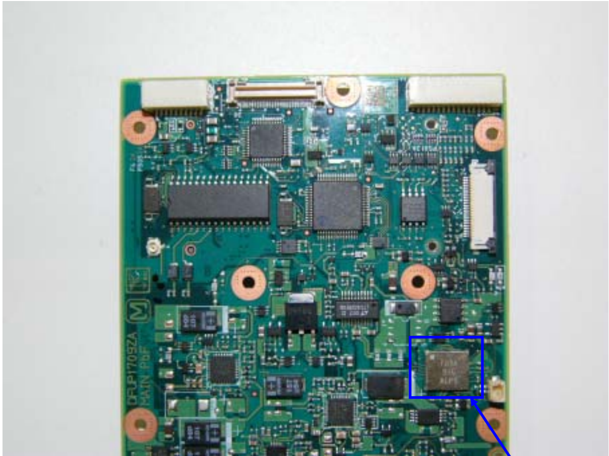
Bluetooth Top View on Main Board
