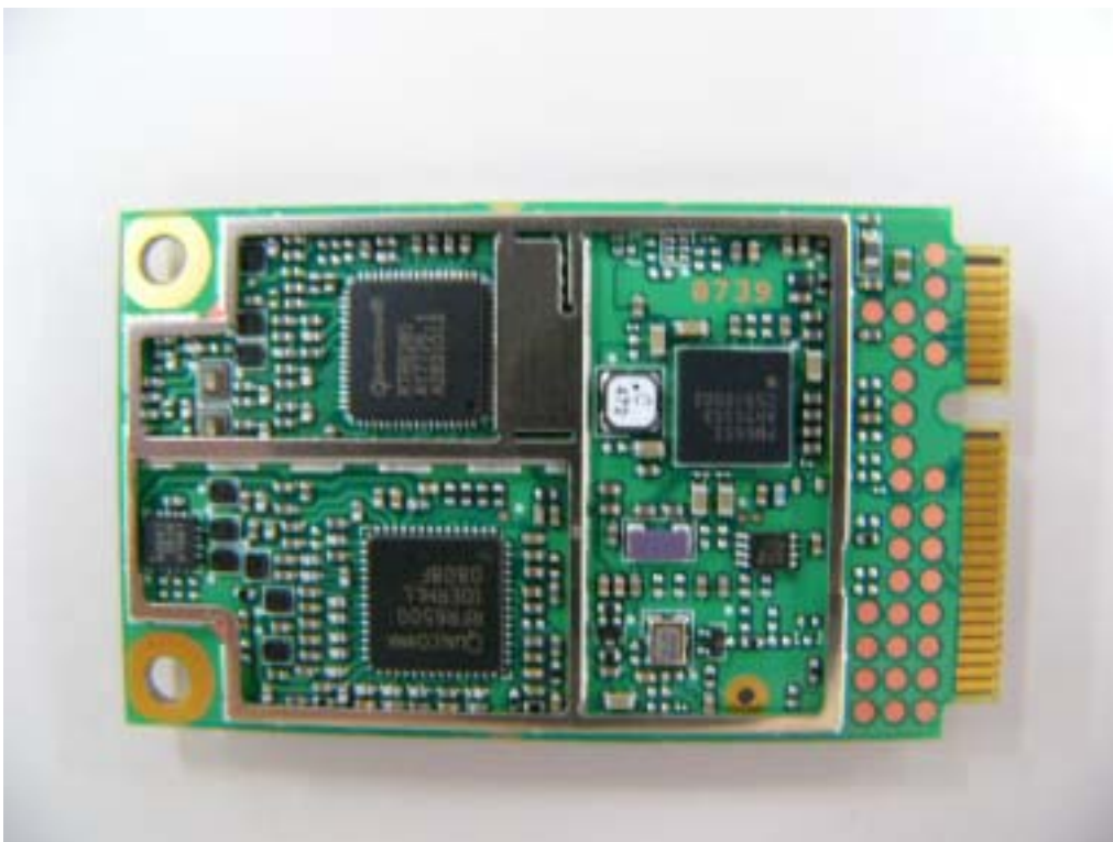
WWAN Module inside Bottom View
