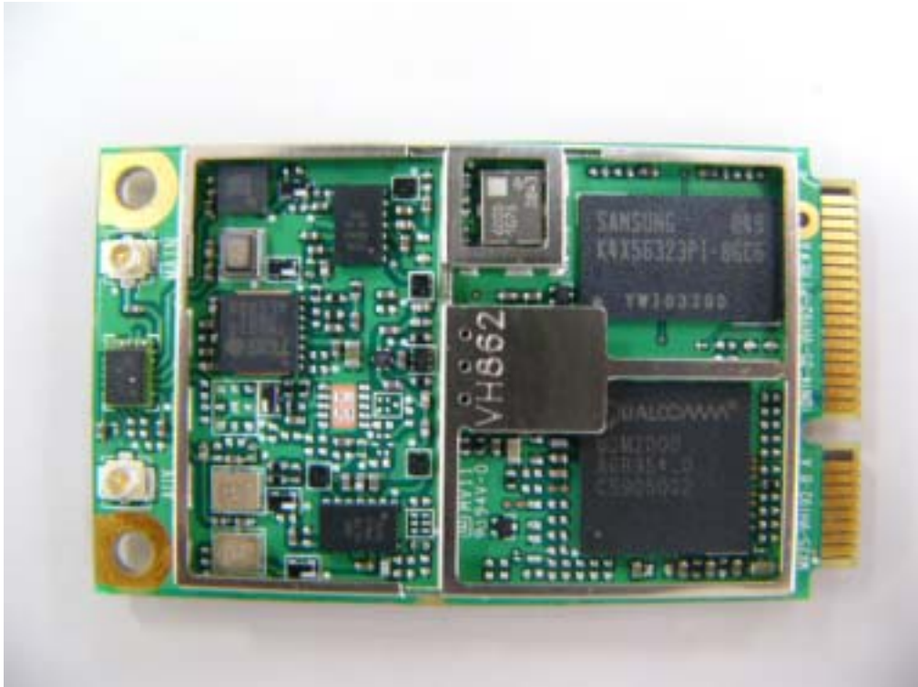
WWAN Module inside Top View
