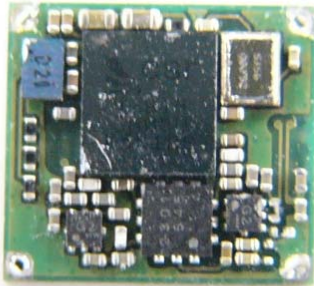
Bluetooth Module inside Top View
