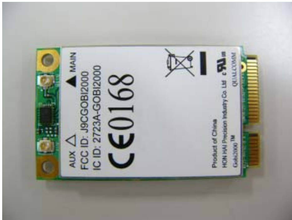
WWAN Module Top View
