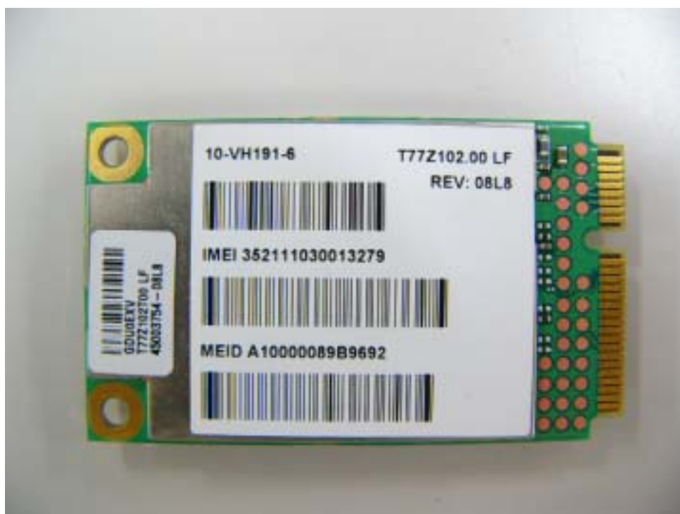
WWAN Module Bottom View
