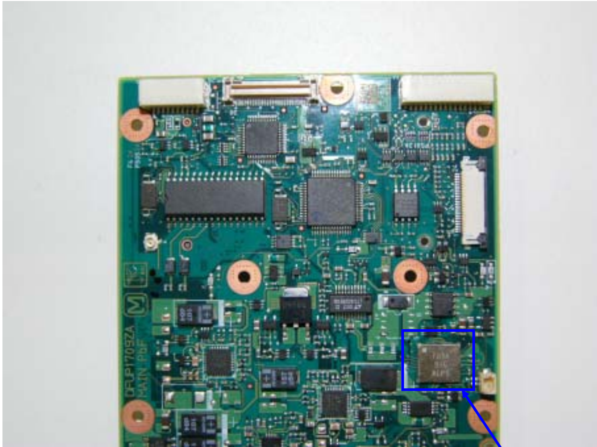
Bluetooth Top View on Main Board
