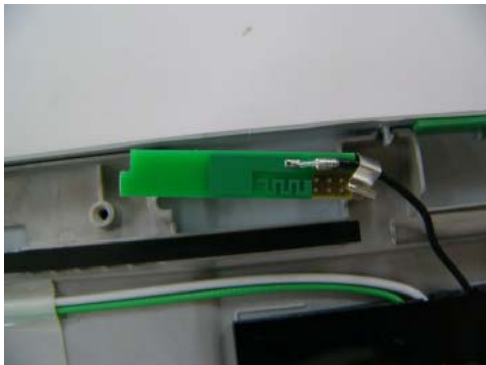
WLAN Main TX/RX antenna bottom view
