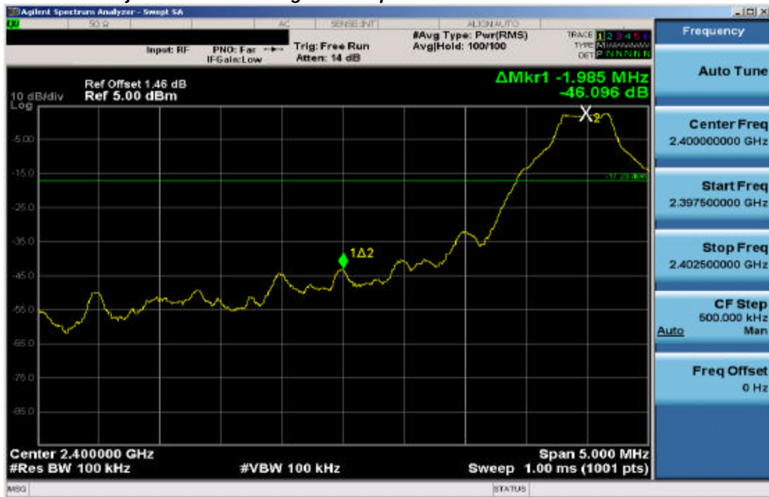
Plot 6-4. Band Edge Plot (Bluetooth – Ch. 0)
