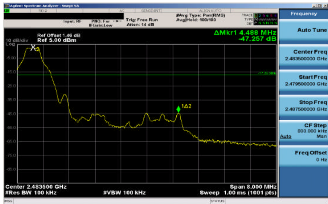
Plot 6-5. Band Edge Plot (Bluetooth – Ch. 78)
