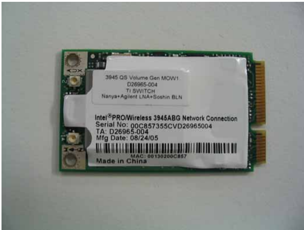
WLAN Top View
