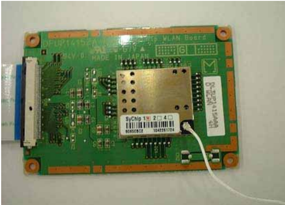
WLAN module (Sychip) on Daughter Board
