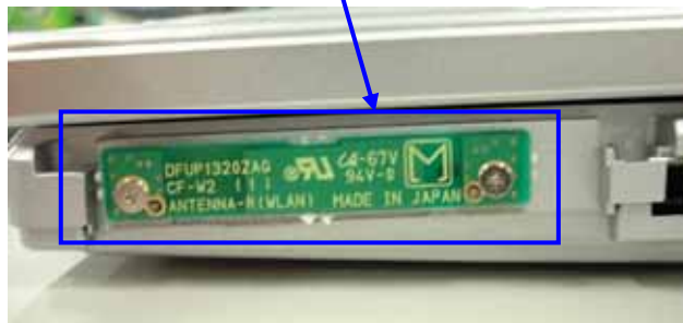
TX Antenna Magnified View
