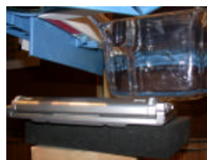
Figure 12.2 Body SAR - Lap Position -
