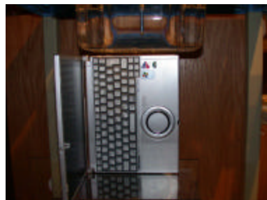
Figure 7.1 Body SAR Laptop and Bystander Configurations
