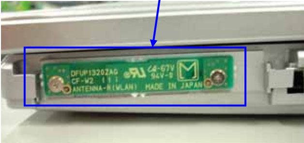
Main TX/RX Antenna Magnified View
