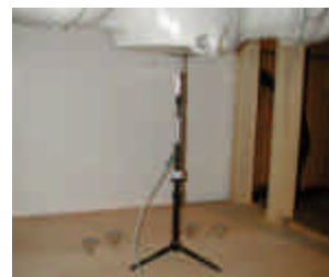
Figure 12.1 Dipole Validation Test Setup
