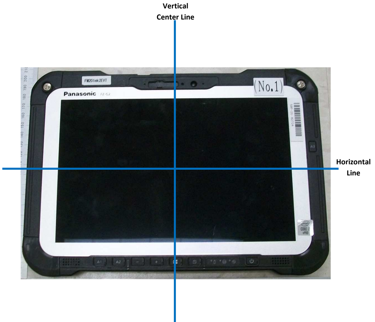
Photograph 6: Handset Vertical and Horizontal Reference Lines
