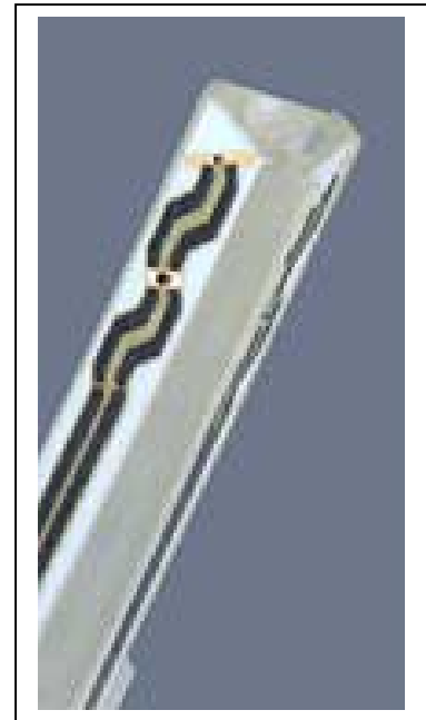
Figure. Inside view of ET3DV6 E-field Probe
