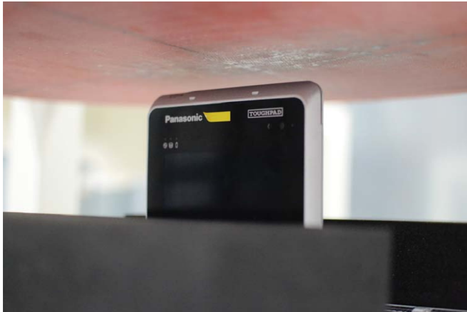
SAR Test Setup Photo 4: Top Edge (Perpendicular) at 1.6 cm
