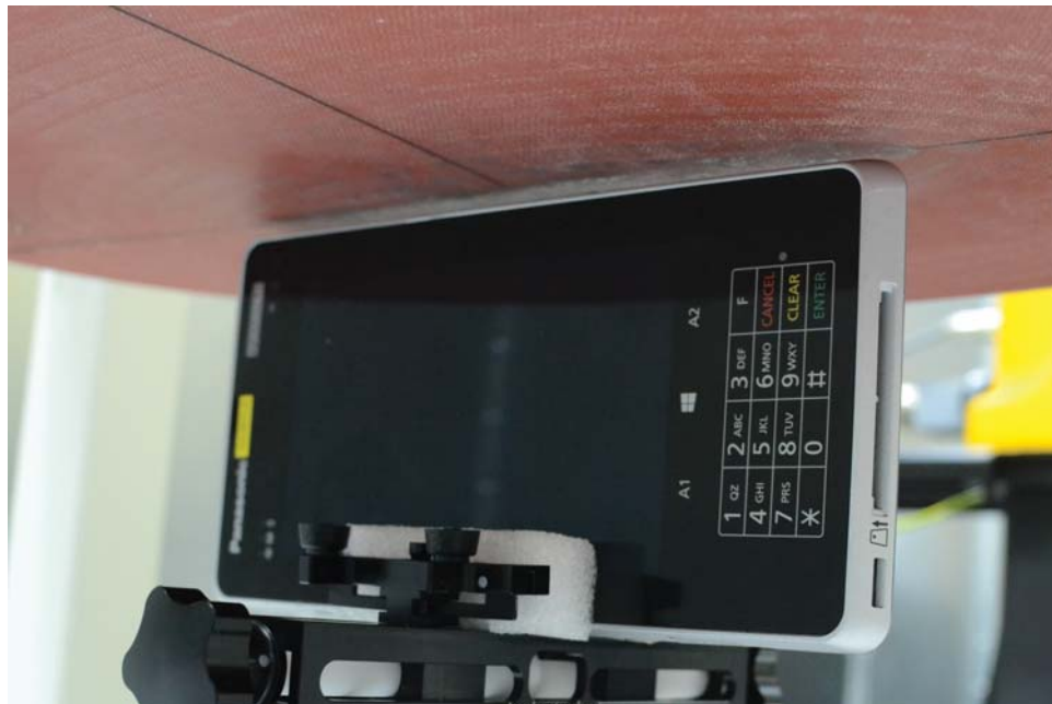
SAR Test Setup Photo 8: Right Edge (Perpendicular) at 0.3 cm
