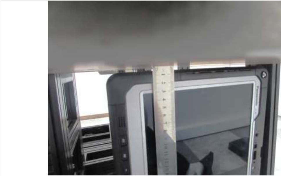
Distance of 5 mm from the EUT
