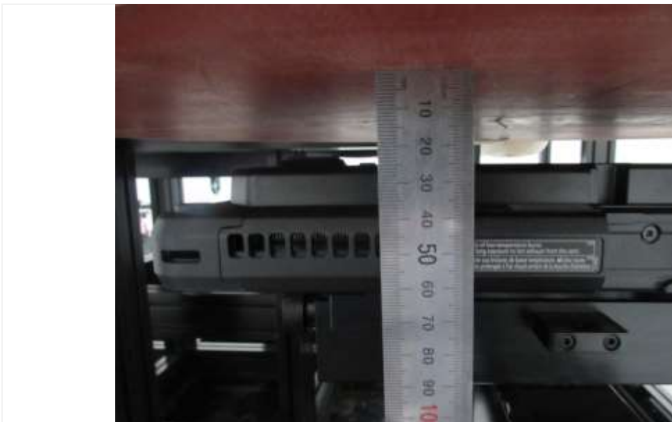
Distance of 25 mm from the EUT
