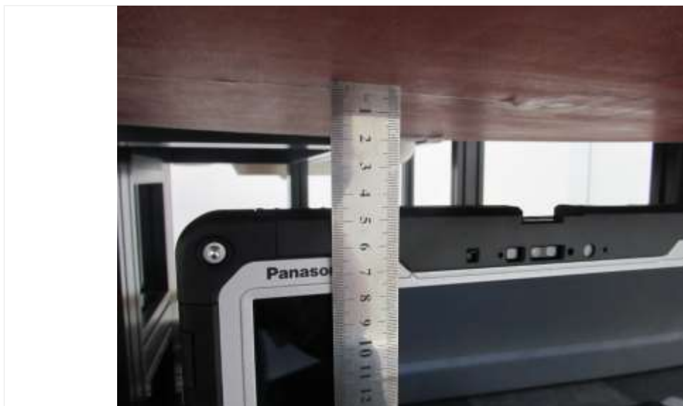
Distance of 45 mm from the EUT
