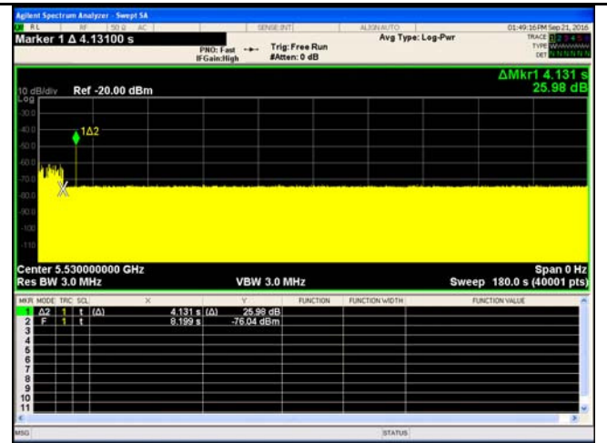
Radar at beginning of CAC – VHT80 – 5530MHz
