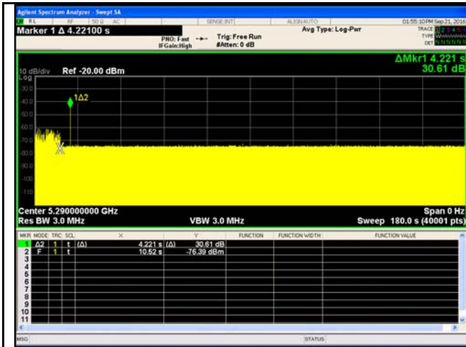
Radar at beginning of CAC – VHT80 – 5290MHz
